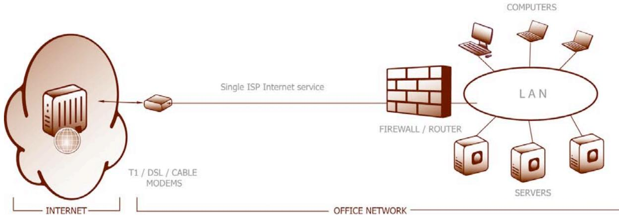
In this scenario, an SMB uses a T1 access line for Internet access. The T1 line may be used for both data access as well as for providing voice communications through a Private Branch Exchange (PBX) system. Because of this, only a fraction of the bandwidth available from the T1 line may be available for Internet traffic. Considering in addition the volume of traffic that may be consumed by incoming spam e-mail, this often leaves little capacity available for useful Internet communications.
