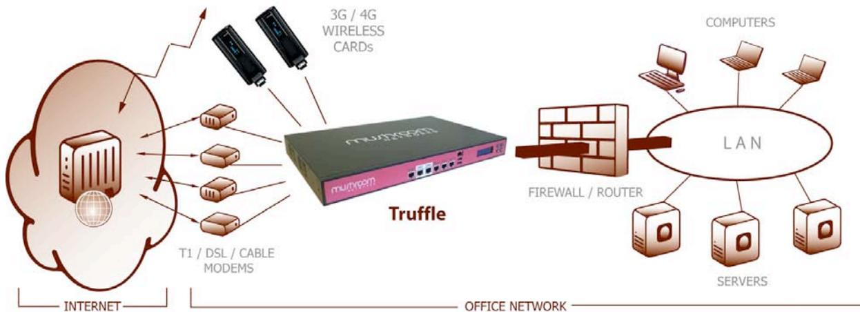
Truffle provides an unmatched level of intelligent aggregation. When peered with another Truffle or the Broadband Bonding Service, Truffle will bond all types of traffic in uplink and downlink directions. In standalone operation, i.e. when not peered with another Truffle, all http downlink traffic will be bonded and all other traffic will be intelligently load-balanced.
